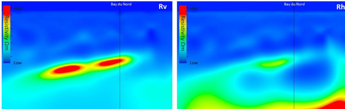
Figure 3: A section from 3D CSEM inversion models, vertical resistivity on the left and horizontal resistivity on the right. The section is crossing the Bay du Nord structure.
