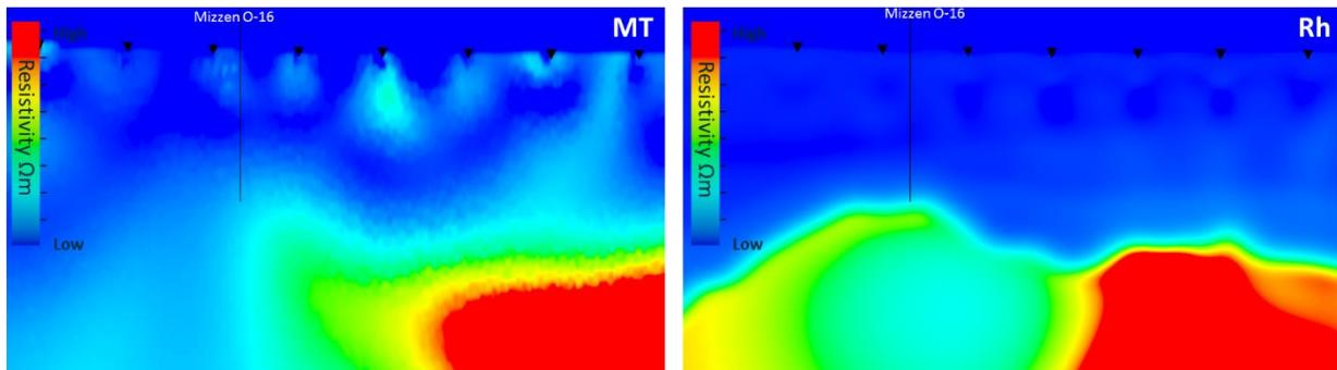
Figure 4: Left: a cross section of 2D MT result. Right: the horizontal resistivity  $R_h$  from 3D CSEM inversion. Both indicate lower resistivity in the Mizzen structure.
