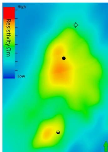
Figure 2: A depth slice through the vertical resistivity model from the 3D CSEM inversion with three Mizzen wells. The results show good correlation with the well data, oil discovery, oil show, and dry well. Warm colors indicate high resistivity and cold colors low resistivity.
