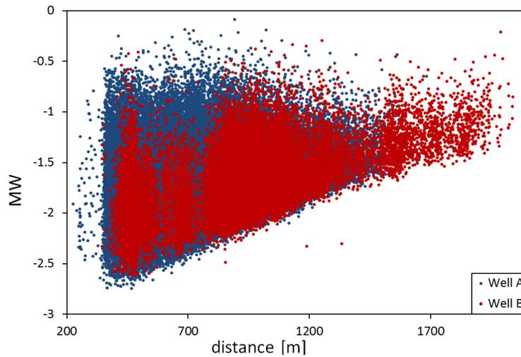
Figure 2: Magnitude versus distance plot for Well A and Well B
