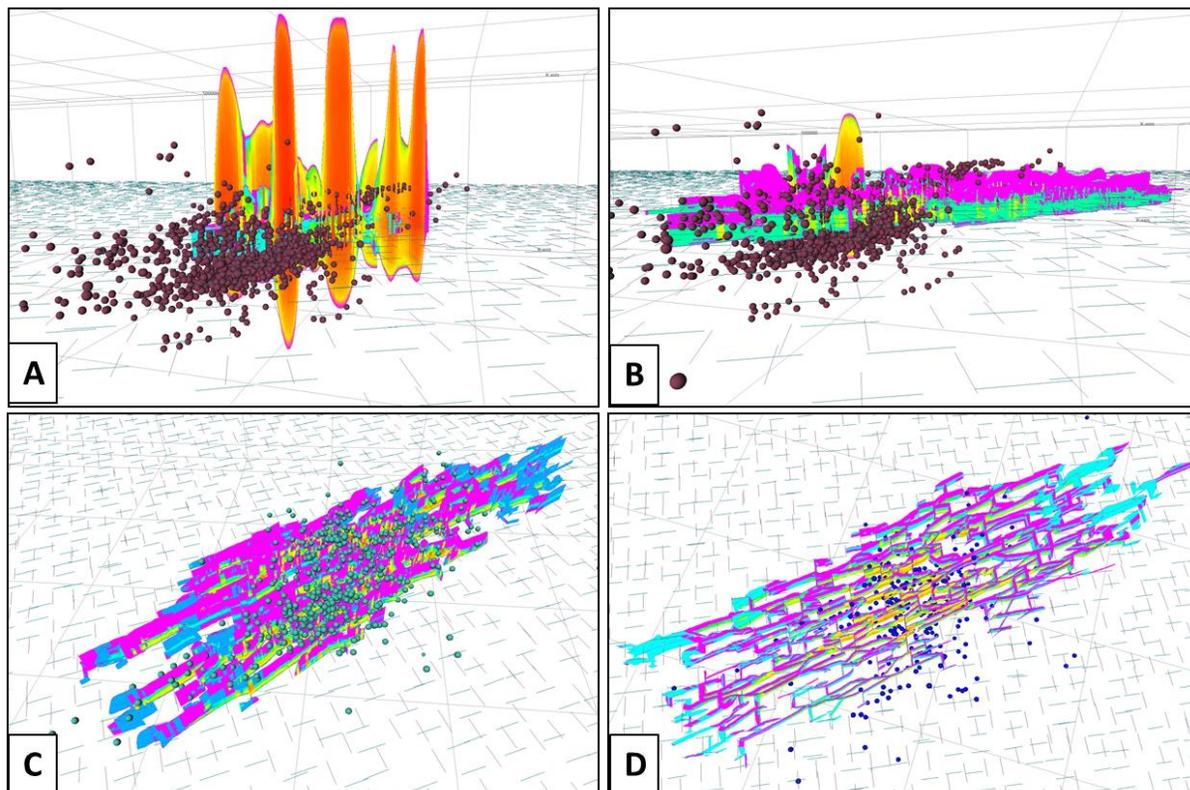
Figure 4: UFM microseismic calibration for different horizontal stress anisotropies. A) Heel stage with overestimated (~5 times) stress anisotropy; B) Heel stage with overestimated (~2 times) stress anisotropy; C) Heel stage-adjusted stress anisotropy; D) Model validation for toe stage. The color of the fracture model represents different fracture width contour. Black “dashed” background lines are the projection of the DFN pattern to the horizontal plane.
