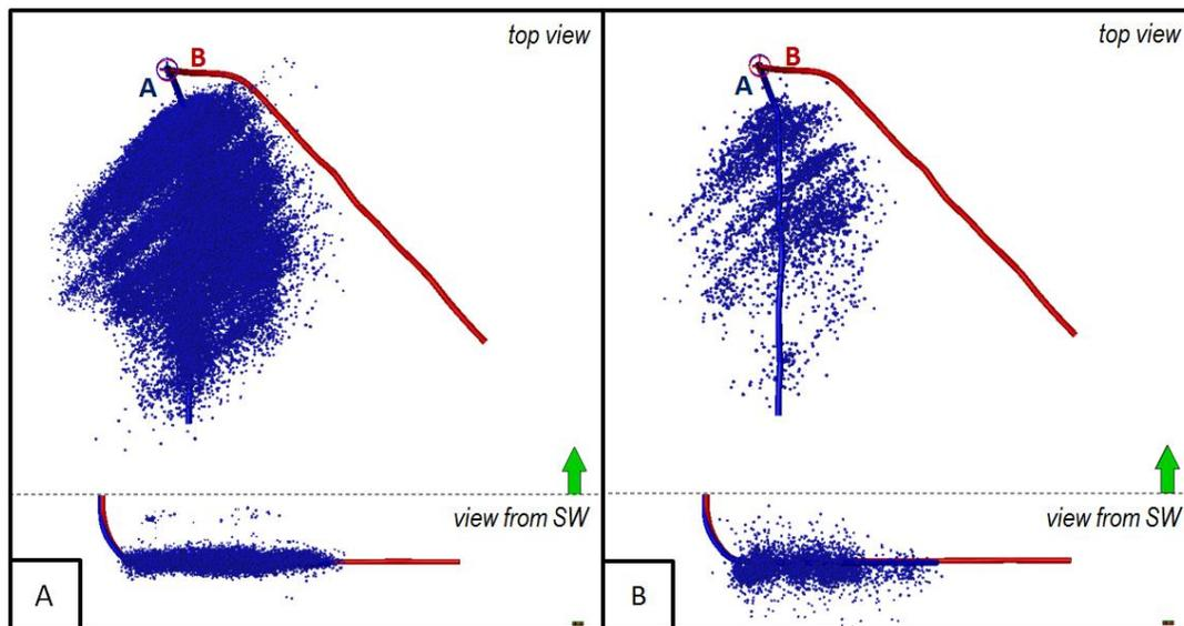
Figure 1: Microseismic events located at Well A. A) With downhole array; B) With surface network.
