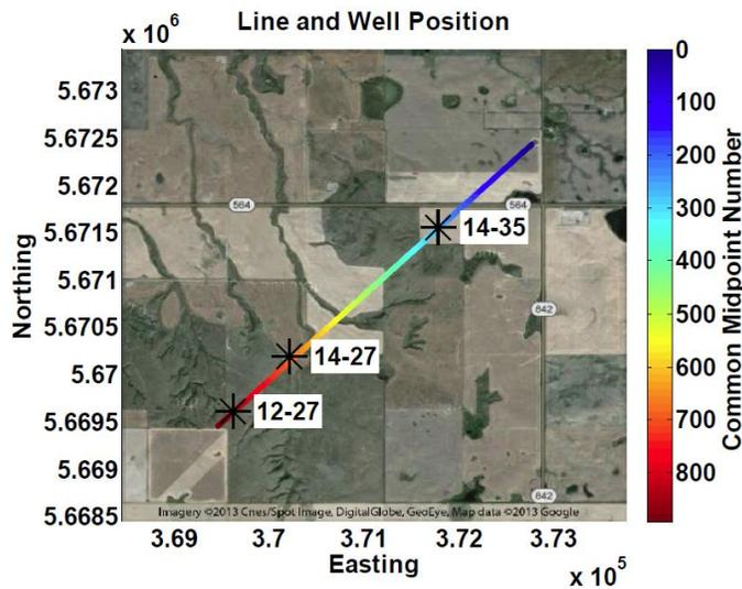
Figure 1: The 4.5km Hussar seismic line is shown along with the locations of 3 wells (from Lloyd, 2013).
