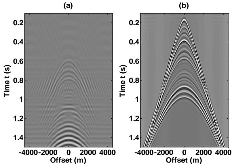
Figure 5: Comparison of prediction output with input. (a) Prediction output; (b) input data.
