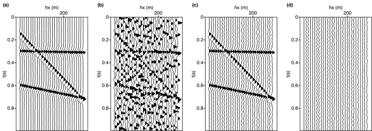
**Figure 1** (a) Synthetic data with linear events in CMPx gather 15. (b) Synthetic data with 3 linear events contaminated with random, spike-like noise to mimic the pseudo-deblended CMP gather. (c) CMPx gather 15 after RPCA de-noising, the SNR has been improved by 11.9 dBs. (d) The estimation error between section (a) and (c).
