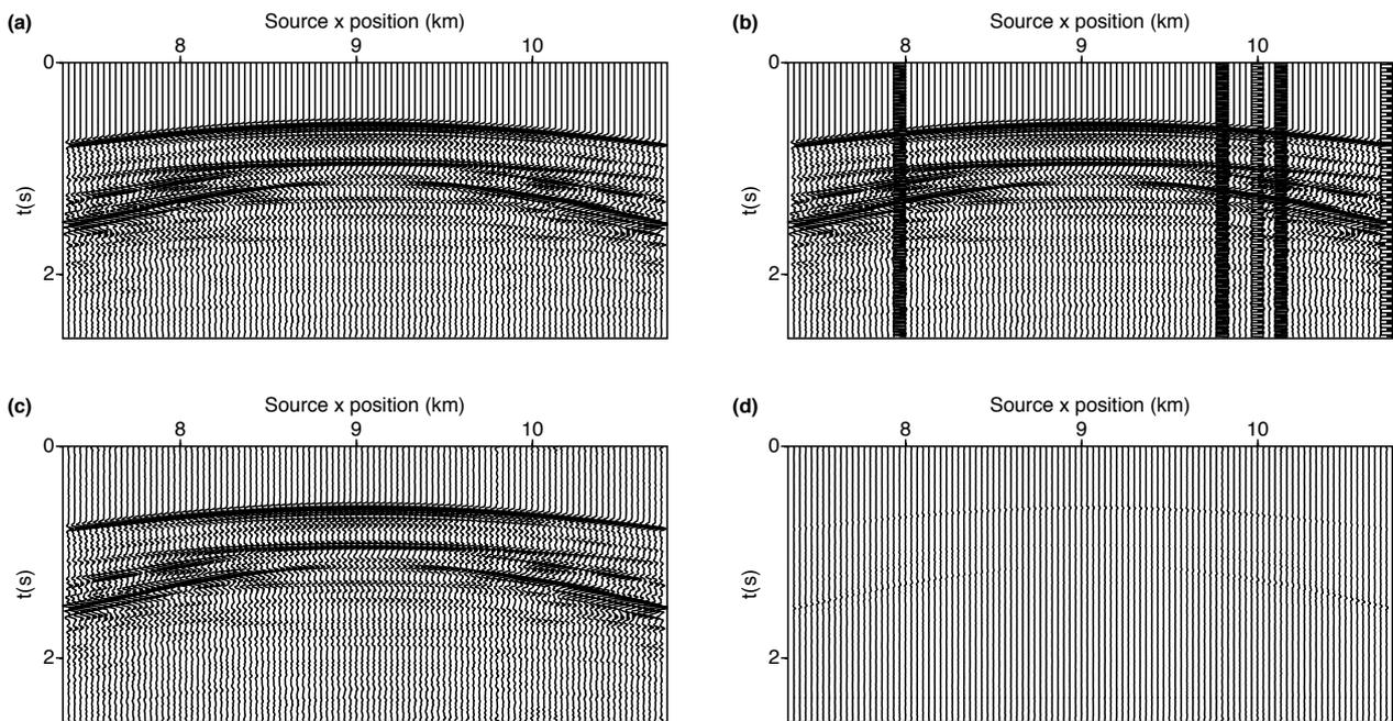
**Figure 2** (a) Centre shot line of the ideal clean common receiver gather of the 3D VSP data set. (b) The centre shot line of the common receiver gather contaminated with erratic noise. (c) The centre shot line of the common receiver gather after RPCA de-noising. (d) The difference between section (a) and (c).
