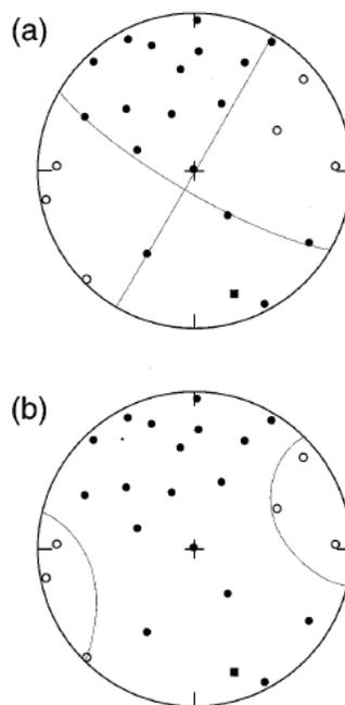
Figure 1. Limitation of the first arrival method. Examples of two different focal mechanisms that fit a high quality dataset. Open and solid circles indicate inward and outward motions, respectively. (a) shows a pure double-couple mechanism, and (b) a mechanism with a large isotropic component. Modified from Julian et al. (1998).
