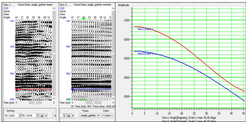
Figure 1. AVO behavior in the base (red) and monitor (blue) seismic surveys at the the reservoir.
