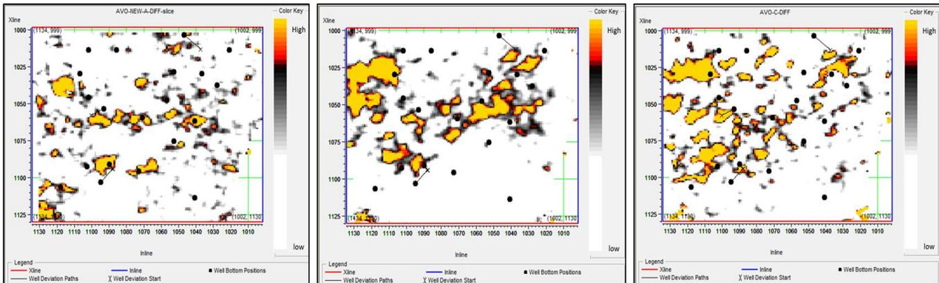
Figure 2. The difference map of AVO parameters A (left), B (middle), and C (right).
