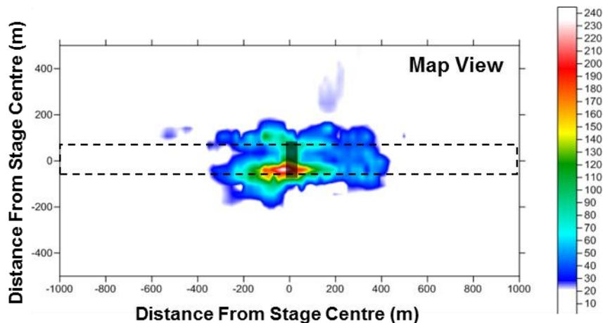
**Figure 2: Cumulative stage map of fracture volume density shows two event trends for a single stage. The black bar shows the interval. This interval is projected away from the wellbore by dashed lines.**
