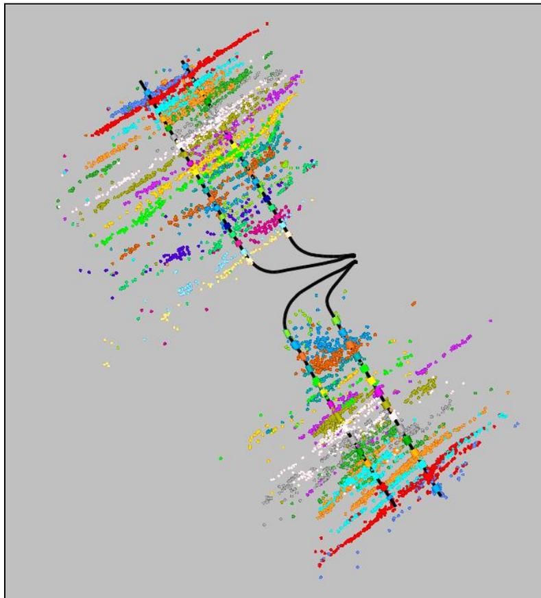
Figure 1: Microseismic results from 4 horizontal wells completed in a Canadian shale play
