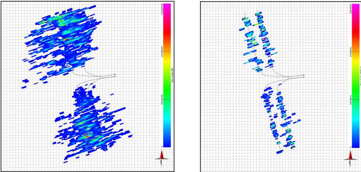
**Figure 3: Total stimulated reservoir volume (left) and productive reservoir volume (right) are shown. Warmer colours represent areas of relative increased fracture permeability.**
