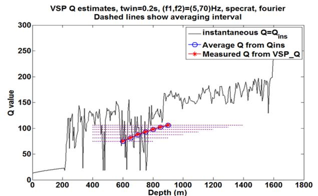
Figure 6: The result of spectral ratio calculations similar to those of Figure 5 except that the downgoing wavefield (not shown) had no multiples or transmission losses. Note that measurements (red stars) now agree with theoretical expectations (blue circles).
