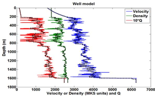
Figure 1: Velocity, density, and intrinsic Q (times 10) curves for 0.5m blocking (colour) and 20m blocking (black dots) as used in this study.
