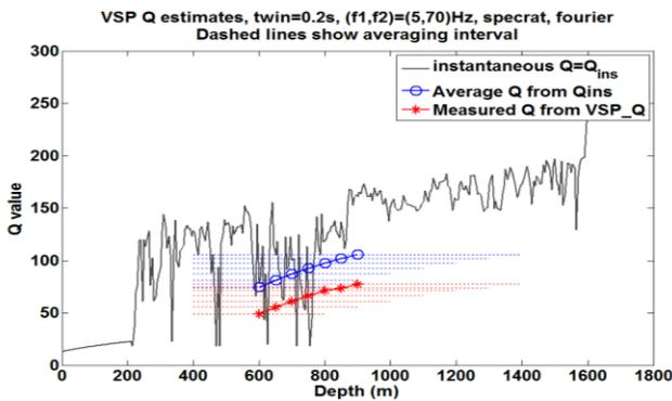
Figure 7: The result of spectral-ratio measurements on the downgoing filed of Figure 8. The internal multiples are confirmed as the cause of the Q measurement bias.
