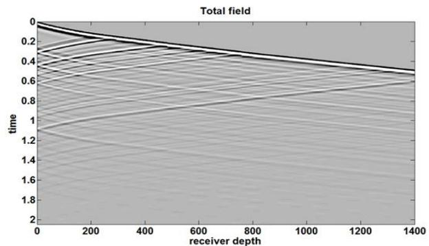
Figure 2: The VSP total field for the 0.5m blocking model shown in Figure 1.
