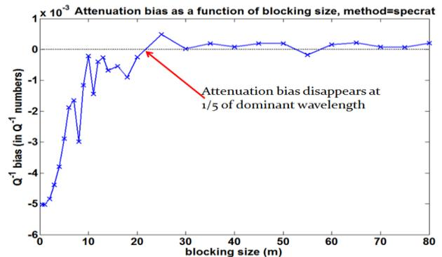
Figure 8: The Q bias, which measures the stratigraphic filtering effect is plotted versus blocking size for a suite of simulations.
