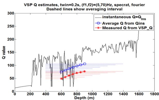
Figure 5: The result of 7 spectral-ratio Q estimates on the downgoing field of Figure 4. Each measurement is indicated by a red star and the associated horizontal line begins at the first receiver and ends at the second receiver. Blue circles denote the expected result of the measurement.
