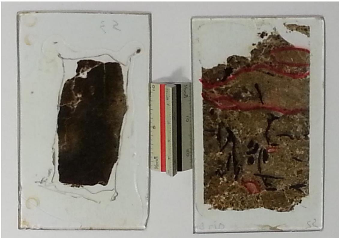
Figure 1: Mammoth-sized petrographic thin sections from oil sands samples obtained using procedure 2. Oil sand samples are from the Hangingstone Section, Upper McMurray Member, and Fort McMurray, Alberta. Thin section on the left is of the Argillaceous Sands and on the right is from bioturbated areas. Trace fossil is captured in the thin section, refer to the area highlighted in red.
