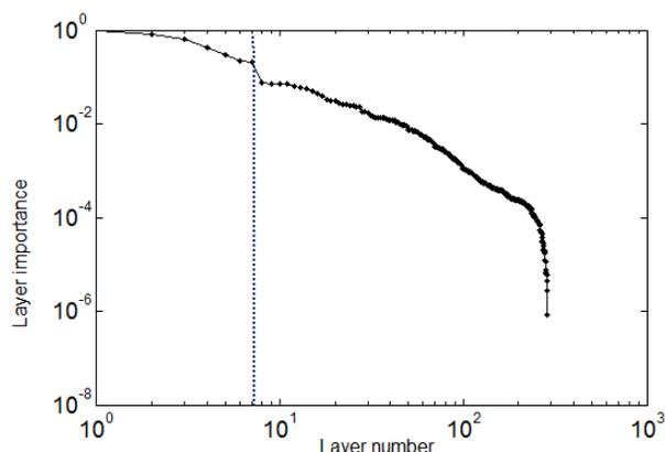
Figure 2- Normalized layer importance for all detected layers by derivative analysis in a decreasing order. Dashed line indicates the significant drop after the 7<sup>th</sup> layer.
