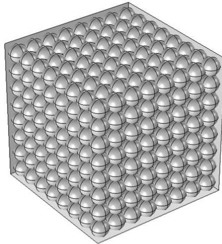
**Figure 1: Generated regular cubical packing of uniform sphere.**
