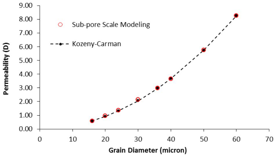
Figure 3: Permeability prediction using Kozeny-Carman equation and sub-pore scale modeling approach.
