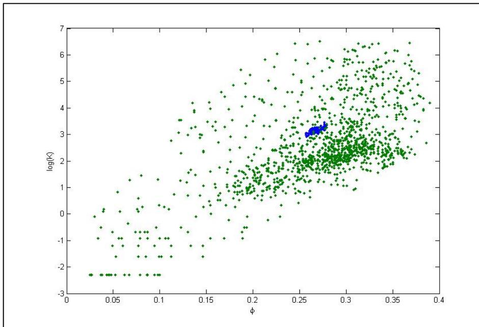
Figure 1 – Porosity vs permeability distributions (original and scaled up)
