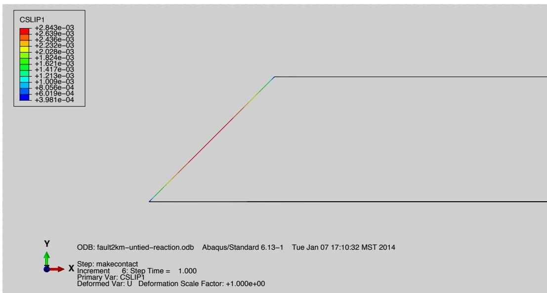
Figure 2: 2.8 m of maximum displacement on fault with perturbation due to hydraulic fracturing. The scale of displacement is km.
