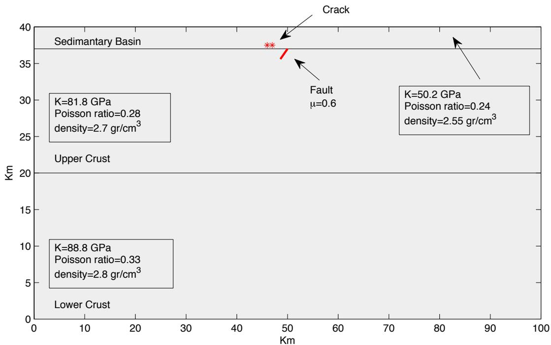
Figure 1: The model which is implemented in ABAQUS, showing 3 layers of 40 km crust. Fault is 2 km long with the 45 degree dipping angle.
