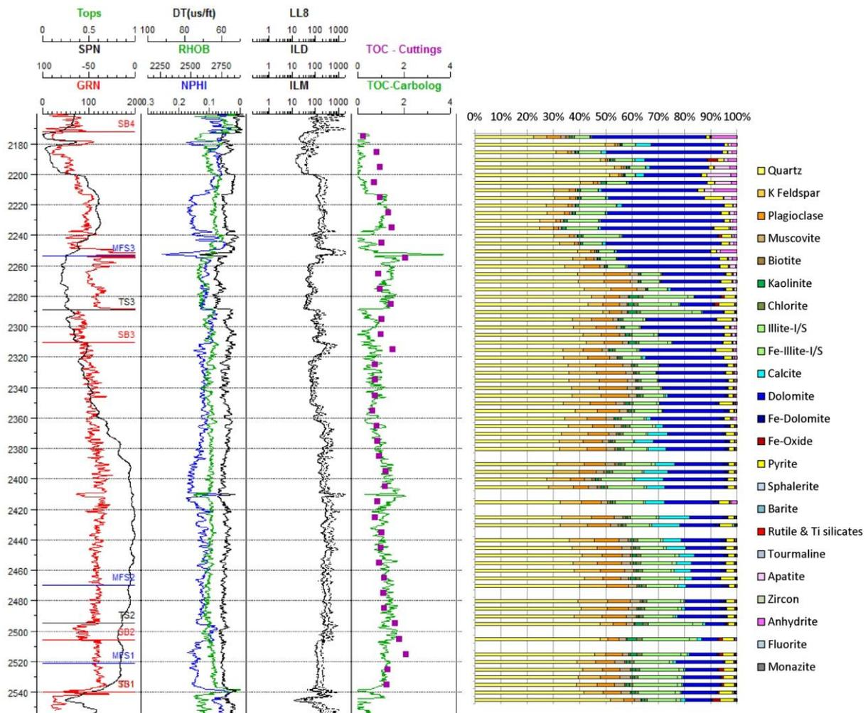
Figure 1: Composite log with TOC Rock Eval data and CARBOLOG estimation as well as bulk mineralogical composition from cutting samples.
