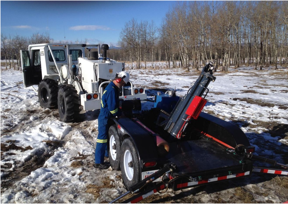
FIG 3. The Envirovibe and the shear wave weight-drop in the field at the Priddis test site.
