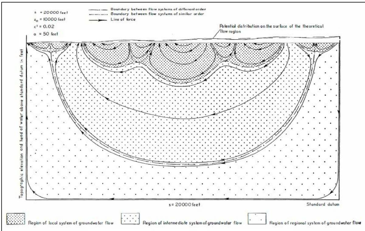
Fig. 4 Analytical model by Tóth [1963]: analytical calculation of groundwater flow systems in a cross-section with homogeneous and isotropic lithology.
