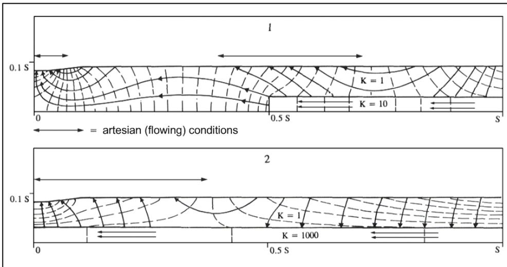
Fig. 6 Mathematical models by Freeze and Witherspoon [1967]: Effect of a buried higher-permeable layer [1,2] upon groundwater flow pattern and location of recharge and discharge areas.
