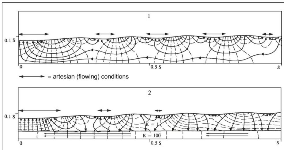
Fig. 5 Mathematical models by Freeze and Witherspoon [1967]: effect of [1] topography and [2] a buried higher-permeable layer upon groundwater flow pattern and location of recharge and discharge areas.
