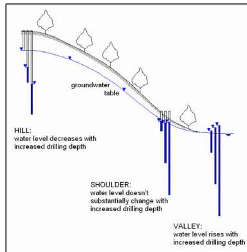
Fig. 2 Schematic depiction of piezometer nests indicating the depth distribution of heads as found by cable tool drilling in the Turner Valley oil field.
