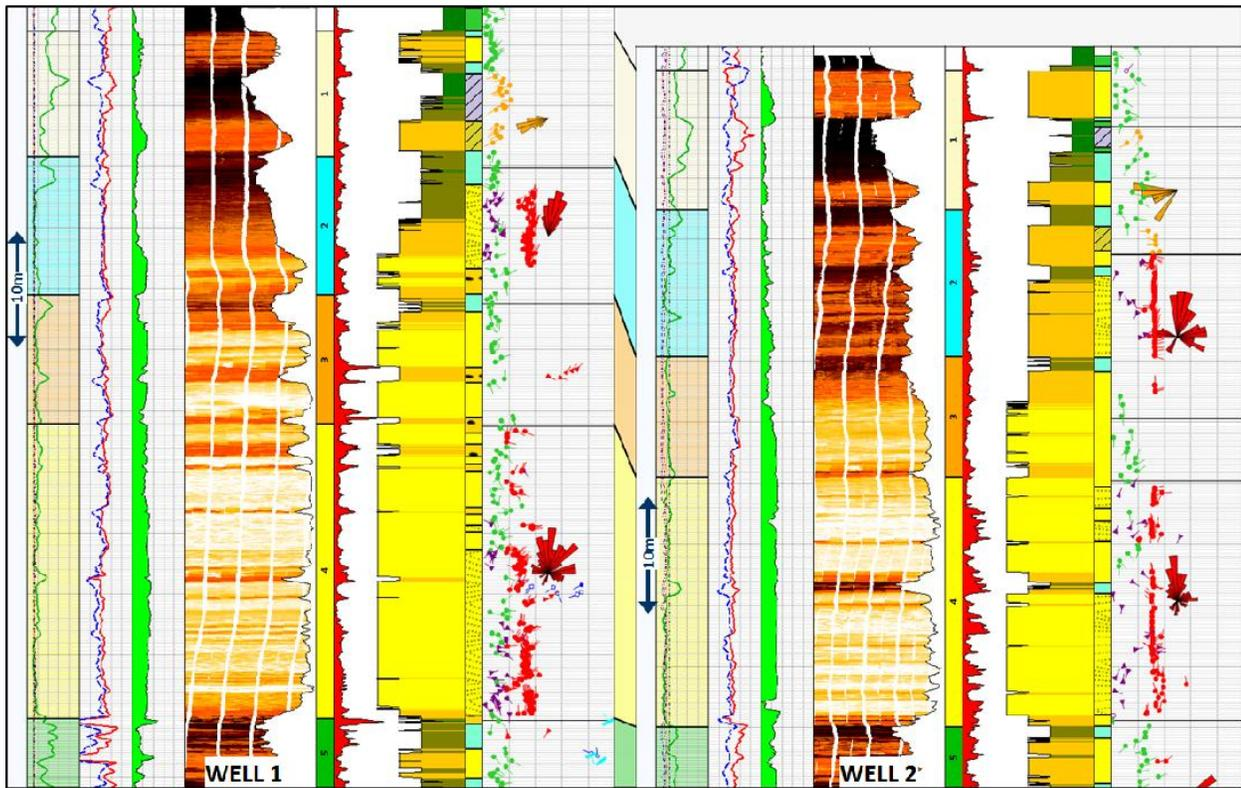
**Fig 1. Example of a comprehensive interpretation from a McMurray reservoir, using microresistivity images and dielectric dispersion data. Track three shows continuous weight percent bitumen values (in green). Track six shows a proxy for sedimentary sorting (in red) and a microresistivity derived electrofacies column. The tadpole data in track eight shows interpreted cross beds and IHS, which help define paleoflow directions and channel thicknesses.**
