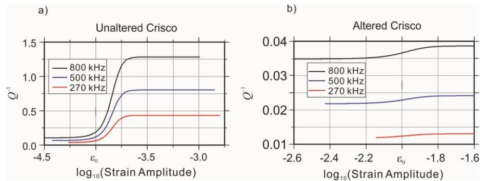
Figure 3. Frequency and strain-dependent nonlinear attenuation. a)  $Q^{-1}$  spectrum of unaltered Crisco with  $\epsilon_0 = 10^{-4}$ , while b) is the  $Q^{-1}$  spectrum of altered Crisco with  $\epsilon_0 = 10^{-2}$ .
