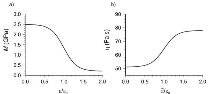
Figure 1. Schematic nonlinear strain-dependent model for unaltered Crisco: a) Strain dependence of the P-wave modulus  $M$ ; b) Dependence of P-wave viscosity  $\eta$  on the combined strain and strain-rate magnitude.
