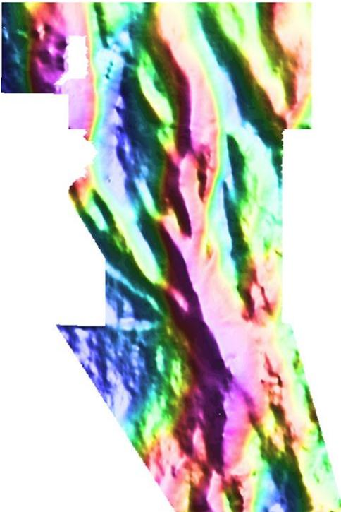
Figure 6: MMR over fault system in Western Australia. Red indicates conductivity highs and blue indicates conductivity lows. Note the numerous branches along the fault system which connect to the central pit in the bottom centre of the map. These branches have gold-bearing potential.
