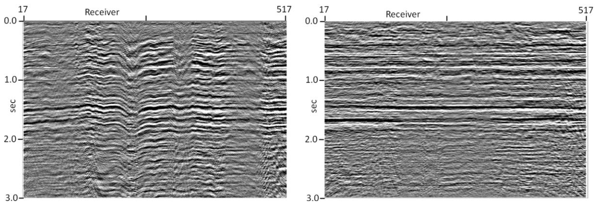
FIG. 5. Common-receiver stack of uncorrected Hussar PS data (left) strongly suggests non-stationary shear statics are required to correct the data. The common-receiver stack on the right shows the result of applying raypath interferometry, which applies non-stationary corrections without altering NMO velocities.
