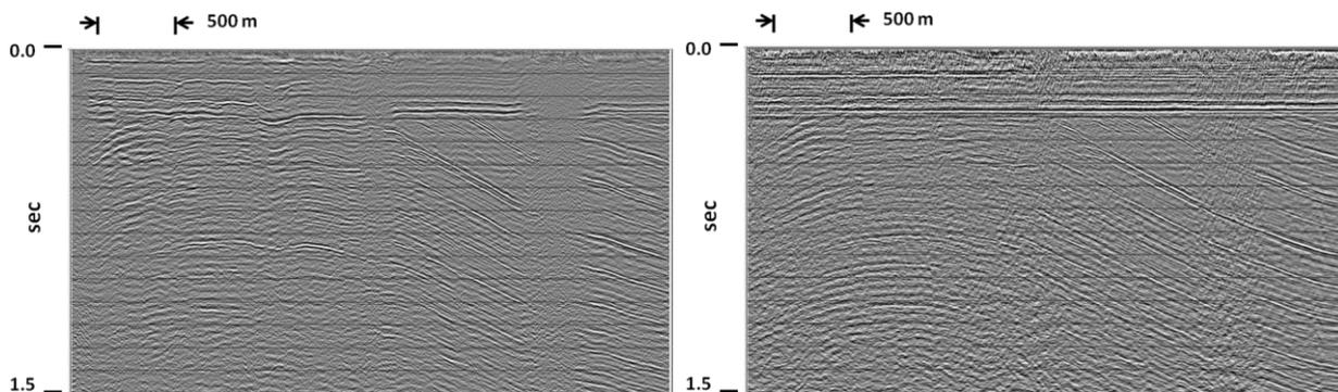
FIG. 1. MacKenzie Delta high-resolution line with visible statics on the brute CMP stack (left). The CMP stack on the right, after raypath interferometry, shows much more near-surface detail, as well as event continuity in the deep structure.
