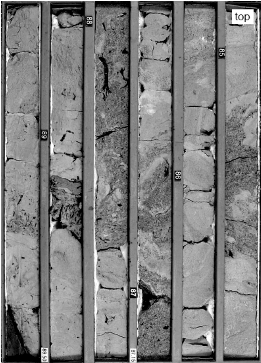
**Figure 2.** Sand dikes developed as numerous intertwined conduits that mobilized fluidized sand upward, often mixed with wall rock. Mud laminar mud ribbons were usually suspended in the flow. Each core box slat is 75 cm long.
