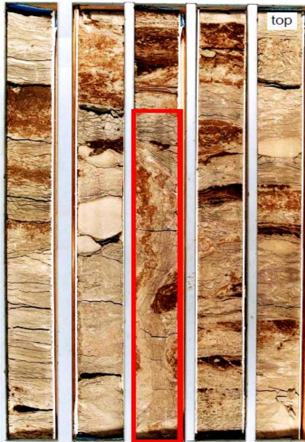
**Figure 3.** Vertical fluidized mud-dominated ribbons (frame) have sinuous to contorted color banded fabrics. The central mud streak passes outward to parallel layers of silt and very fine sand. Each core box slat is 75 cm long.
