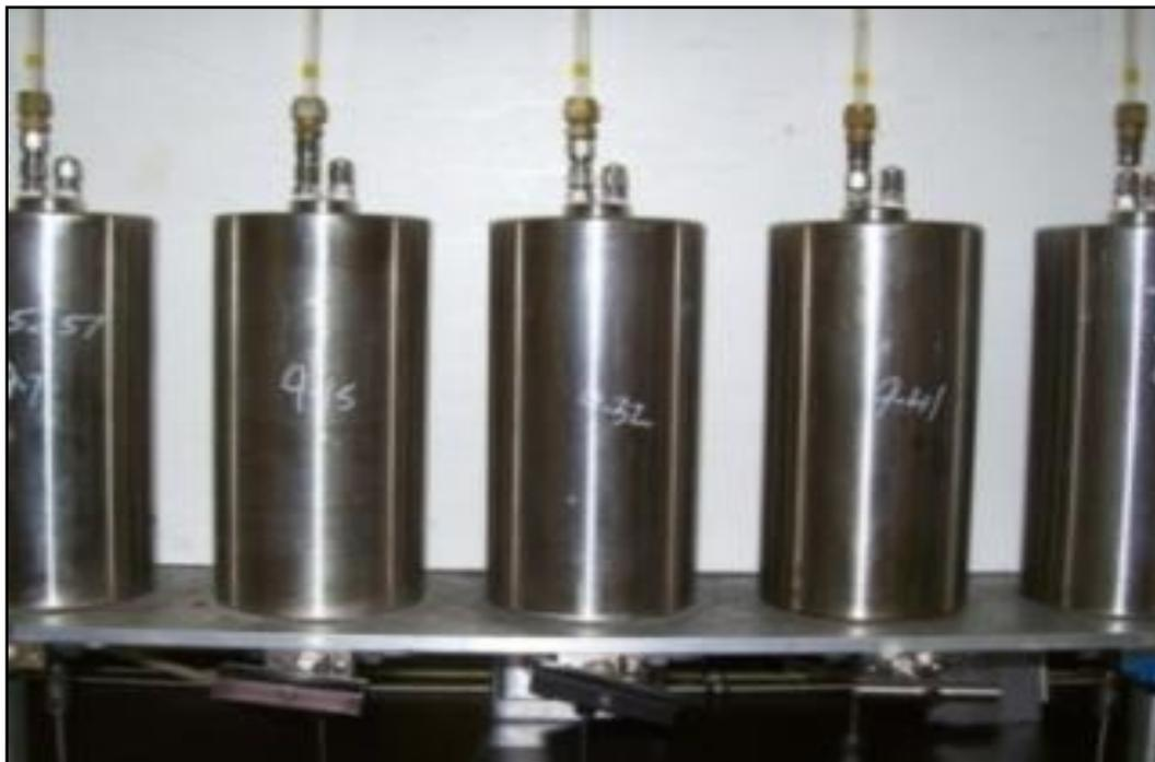
Figure 6: Hydrostatic Test Cells
