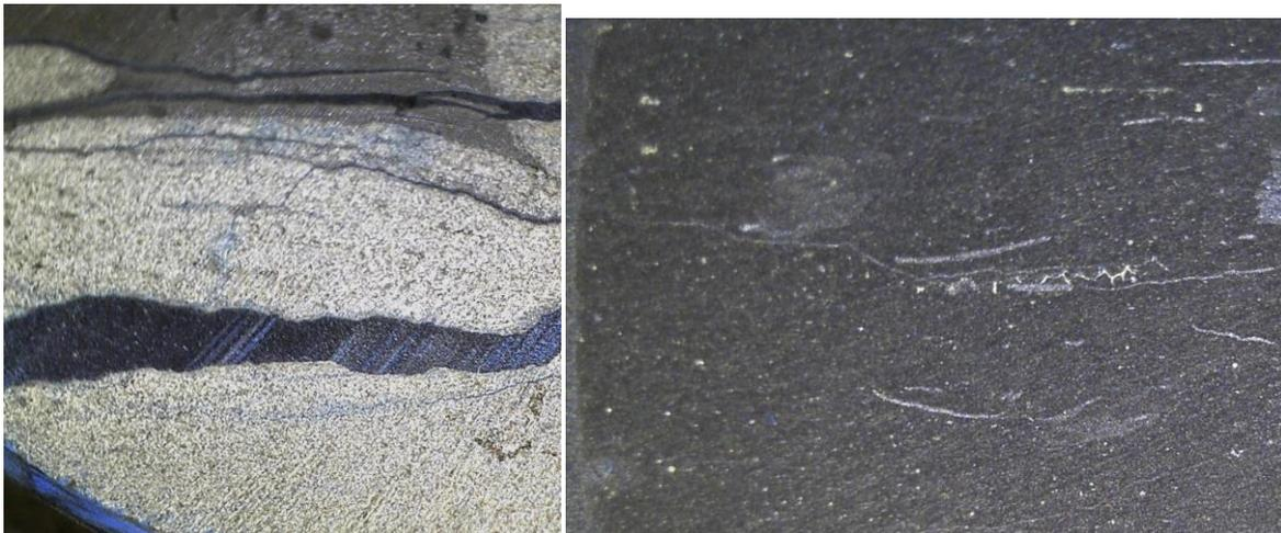
The above photographs show epoxy injected into existing fractures without entry into the surrounding pore structure. Left: a tight gas sand example. Right: a shale sample. Epoxy injection pressure is “matched” to the pore structure: 20 psi was used on the tight gas sand sample and 1000 psi was used on the shale sample.
