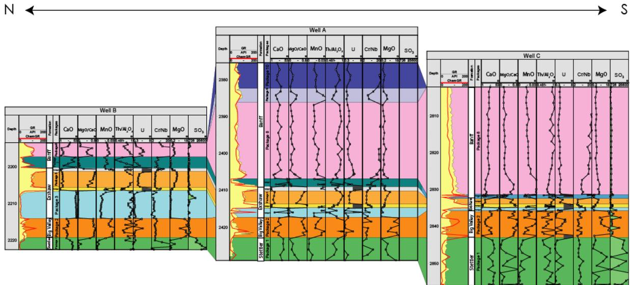
**Figure 1.** Chemostratigraphic characterization and correlation of three vertical wells of the Alberta Bakken Petroleum System (ABPS) of SW Alberta.
