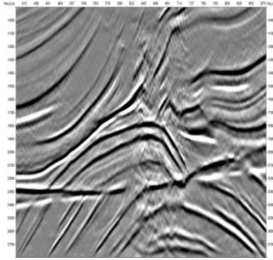
Figure 4b. PSDM image obtained from the ZOMF enhanced gathers. Places of non-hyperbolic traveltimes surfaces are deteriorated.
