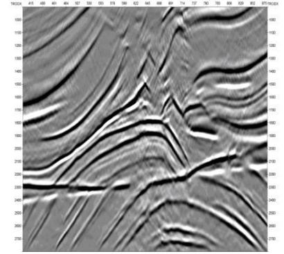
Figure 4c. PSDM image obtained from the COMF enhanced gathers. The image is very close to the correct one shown in figure 4a.
