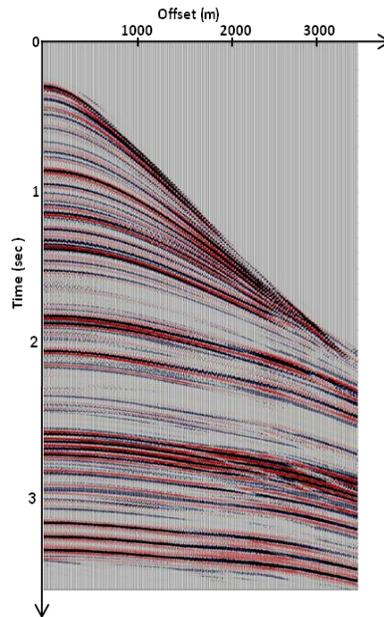
Figure 3a. The same CMP gather as shown in Fig. 2b after ZOMF signal enhancement. Events in the deep part are deteriorated.
