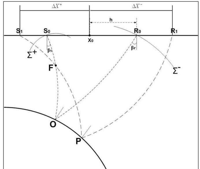
Figure 1. Schematic representation of the common-offset multifocusing.
