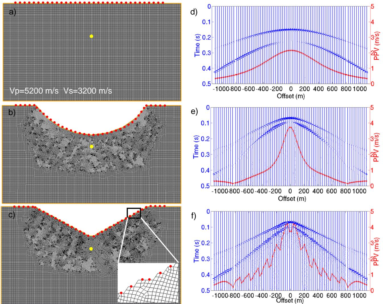
Figure 2: Open-pit mine simulations; the left column illustrates three meshed models with increasing complexity of surface topography, and the right column shows their corresponding calculated peak particle velocity (PPV) and synthetic seismograms; red dots indicate the receiver locations, and yellow spots highlight the source locations; sizes of all models are approximately 2616 m X 1427 m.
