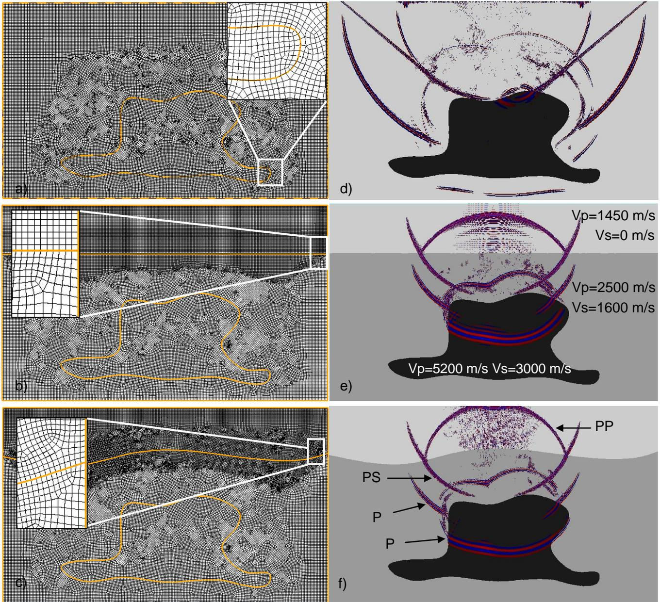
Figure 1: Subsalt simulations; the left column shows three meshed models with increasing complexity, and the right column shows their corresponding SEM simulation snapshots at  $t=0.74$  s; the sizes of all models are 4000 m X 2400 m.
