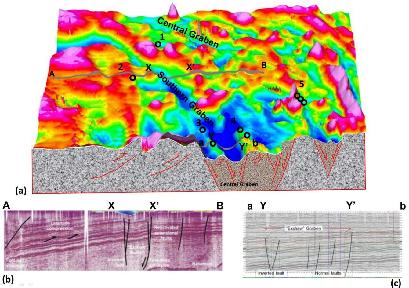
Figure 3 Three dimensional diagram of High Resolution Magnetic data and regional seismic over the Canadian portion of the Exshaw/Big Valley play area. The circles represent Exshaw-Big Valley wells that produced over 250 bbl/d.
