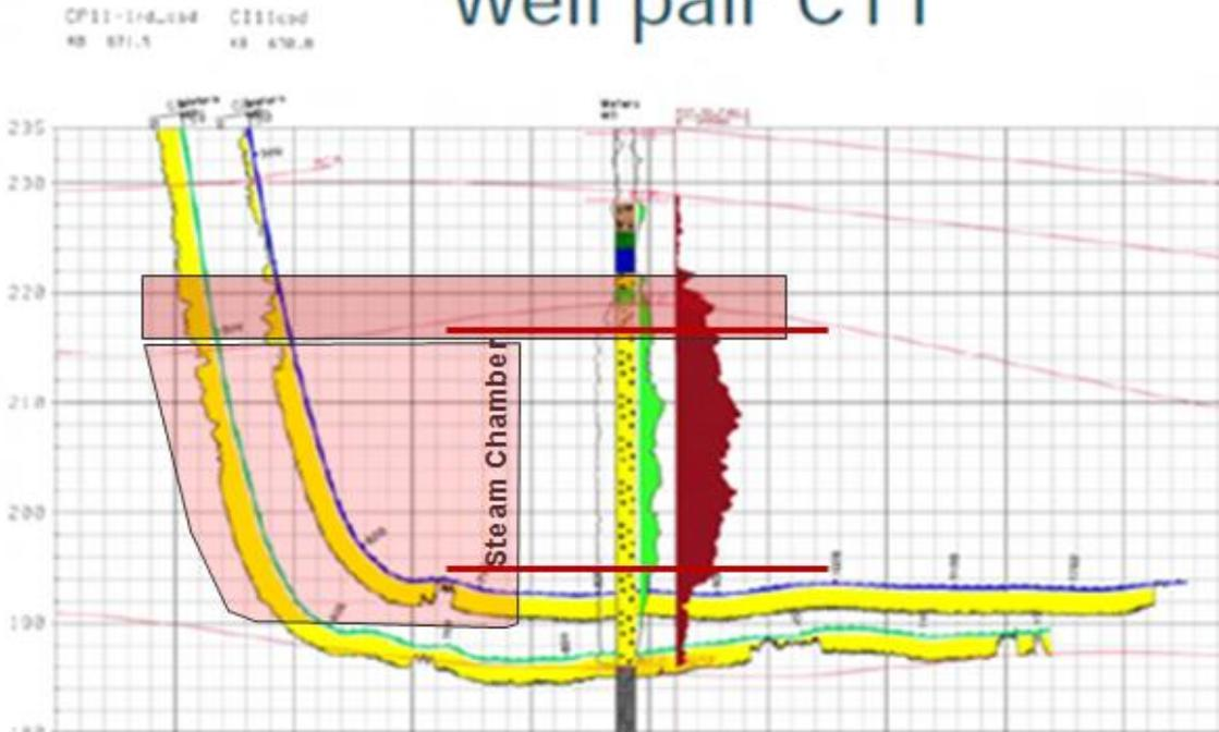
Figure 6. Observation well B6-22, Well Pair C11, illustrating production due to conductive and radiant heating. Additional recovery from the heel area of this well is verified by time-lapse seismic. Modified after the Cenovus 2011 annual report to the ERCB.
