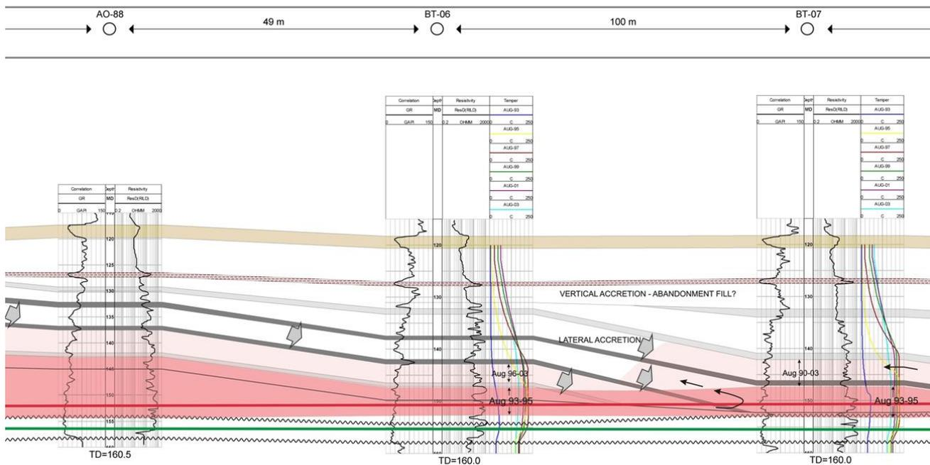
Figure 1. UTF Phase B steam temperature data for the middle portion of the B2 SAGD well pair, illustrating the limited steam-chamber growth due to mud-dominated IHS beds 75 cm thick, but with a lateral extent of 160 m x 300 m. Note the proposed down-slope displacement of conductively heated bitumen (large, grey arrows) along sand-dominated IHS beds and subsequent production. Source: Strobl, 2012.
