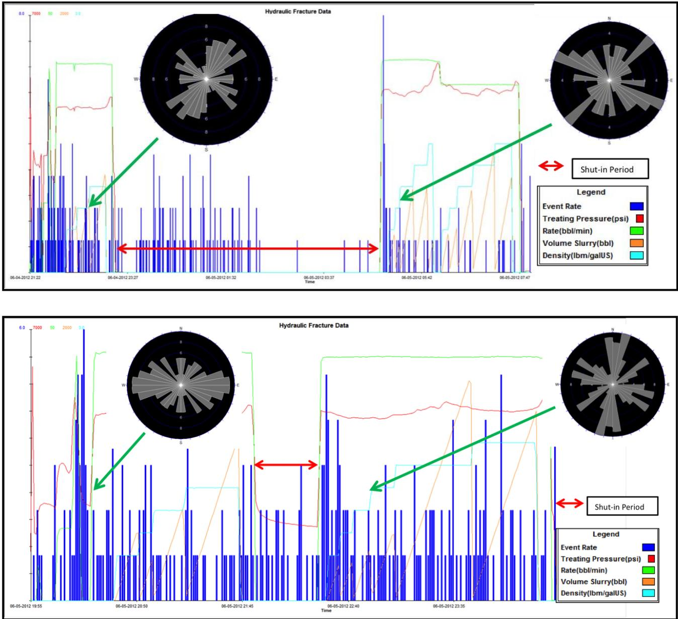
Figure 3. Top. Well 2, Stage C cyclic injection program (hesitation fracture) with a 24 hour shut-in (flow back) period. Bottom. Well 2, Stage E cyclic injection program (hesitation fracture) with a shortened shut-in (flow back) period.
