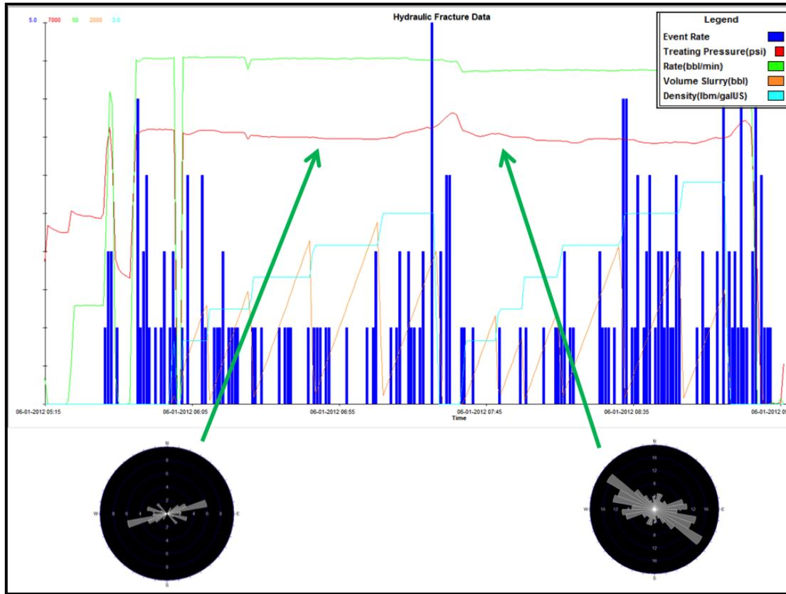
Figure 2. Early Well 2 stage showing re-orientation of the fracture set as a result of injection pressure changes (red) during the stimulation.
