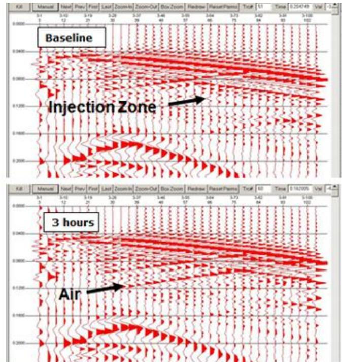
Figure 3) Single shot recordings before (top) and after three hours of air injection (bottom)
