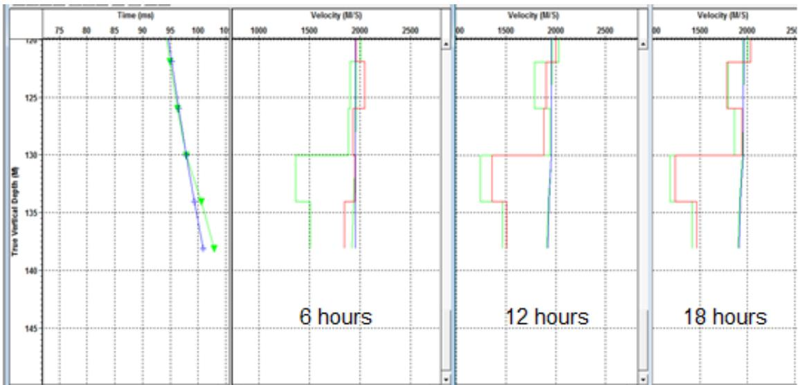
Figure 6) arrival times before injection (blue) and after 6h (green); 2) interval velocity before injection (red) and after 6h injection (green); 3) interval velocity after 6h injection (red) and after 12h injection (red); 4) interval velocity after 12h injection (red) and after 18h injection (red).
