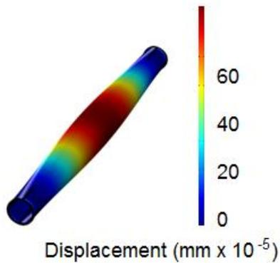
**Fig. 4** –A COMSOL model showing an exaggerated view of fundamental-mode displacement of a 2 m long steel pipe fixed at the ends after excitation by an internal acoustic source.
