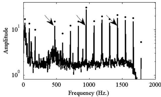
**Fig. 2 –** The frequency spectrum from trace number 1 in Figure 1. The fundamental mode occurs at ~ 467 Hz. (indicated by the left arrow). Overtones (arrows) and other spectral peaks are evident.
