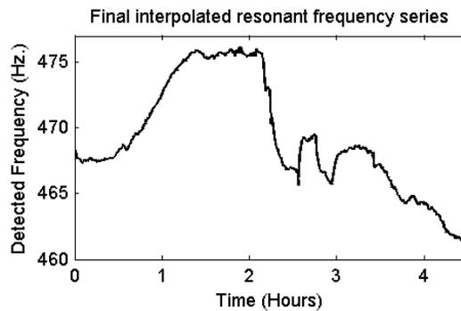
**Fig. 3 –** The detected frequency vs. time for the fundamental mode in Figure 2. This plot is the median filter for the detected fundamental frequency from the 33 geophones that recorded the central Alberta dataset. The observations are robust; about 100 samples out of 645000 values before the median filter fell outside of a 0.2 Hz corridor around this curve.
