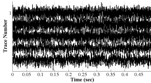
**Fig. 1 - A** 0.5 second window of five traces of vertical-component data from a 2010 microseismic survey in central Alberta. The borehole geophones are clamped 12.37 m apart.
