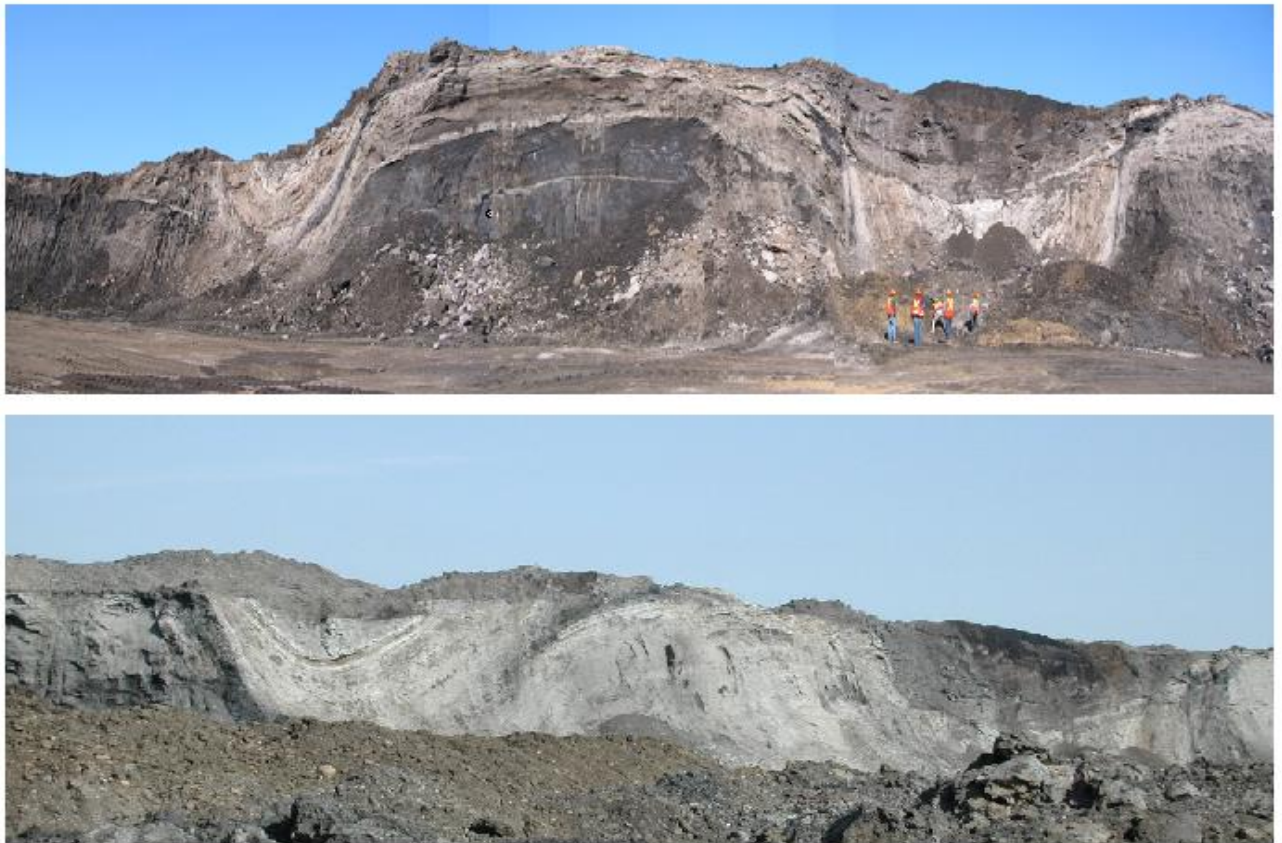
Figure 1. Two examples of lower McMurray sinkhole sags exposed by bench cuts in the Aurora mine in the south-central Bitumont trough. Each mine bench has a 12-15 m high cut face. These double sag structures have kaolin paleosol beds. Upper photograph courtesy of Syncrude; lower photograph courtesy of the Alberta Geological Survey.
