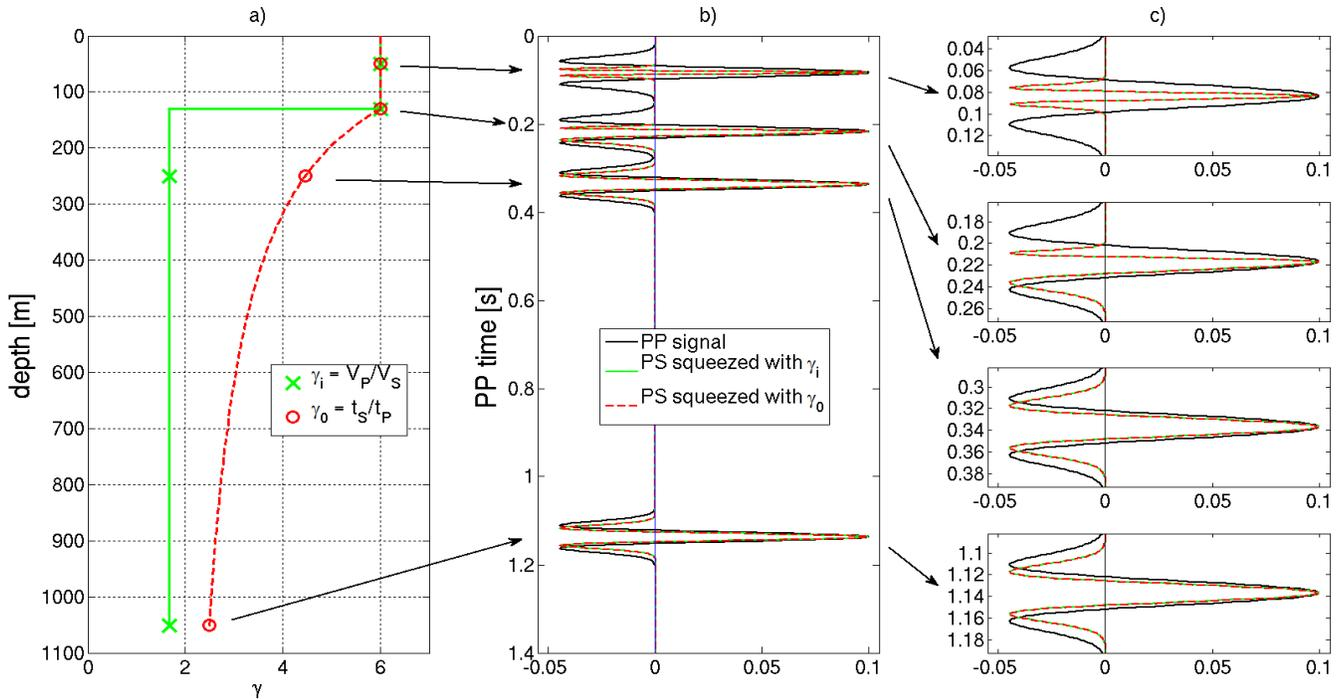
Figure 1: (a) Interval and average  $V_p/V_s$  values in depth for a simple model. The locations of four reflectors are indicated by symbols. (b) A PP trace (black line), a PS trace compressed to PP time by a method that uses interval  $V_p/V_s$ ,  $\gamma_i$  (green line), and a PS trace compressed to PP time by a method that uses average  $V_p/V_s$ ,  $\gamma_0$  (dashed red line). (c) Close-ups of each of the four events in (b).
