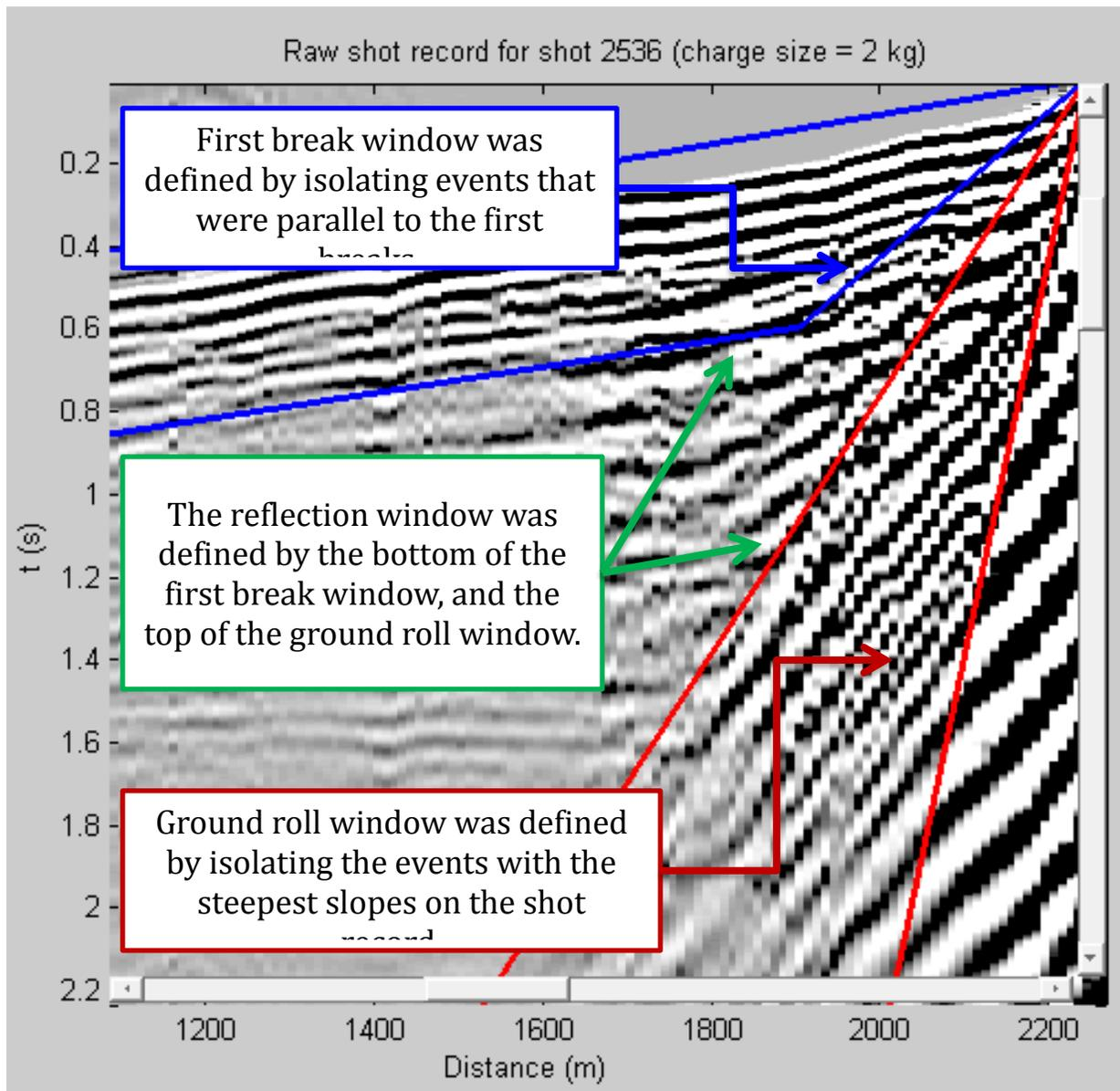
Figure 2: Criterion used to isolate each component from the rest of the shot record.
