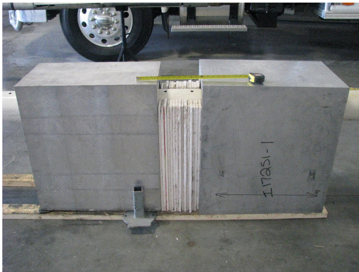
Picture 1: Calibration Blocks (Magnesium on Left) with ~190 mm Gyprock.
