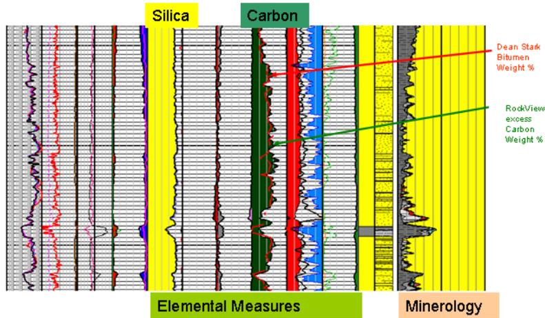
**Figure 2 Five Well Comparison -** of elemental excess carbon weight from spectroscopy tool to Core
