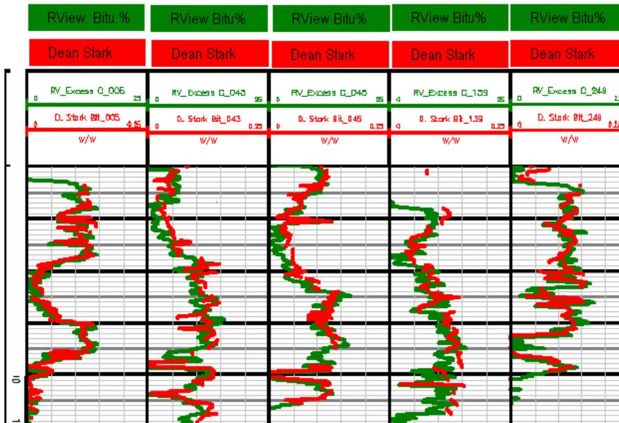
**Figure 3 RockView and NMR** – the combination of these measurements permit identification of fluids saturations such as bound water%, free water%, total bitumen%, lighter hydrocarbon % and gas saturation %
