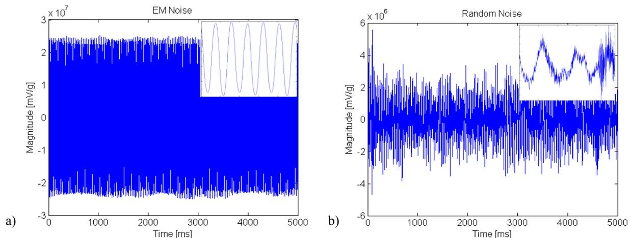
Figure 1: (a) EM noise at 60Hz picked up by a sensor. (b) Random background noise picked up by a sensor. Both insets show a zoom-in window of 0 to 100ms.
