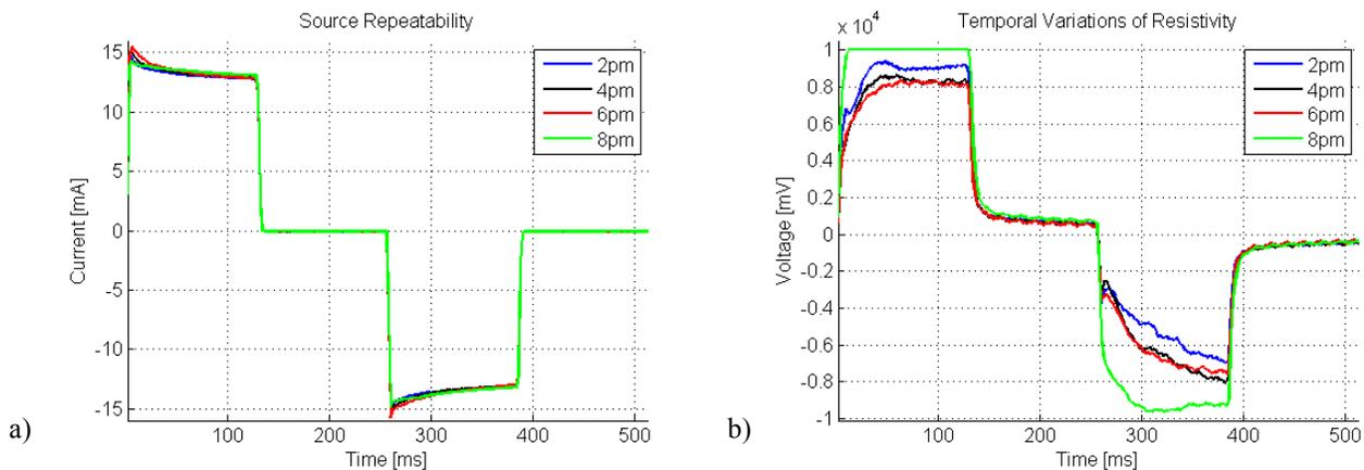
Figure 5: (a) Current injection. A bipolar square wave is used as the controlled source. The waveform is stable and is ideal for repeated measurements. Readings are taken every 2 hours. (b) Voltage response. Transients are observed when the source is changed abruptly. Recorded signals are different, indicating changes in the formation over time.
