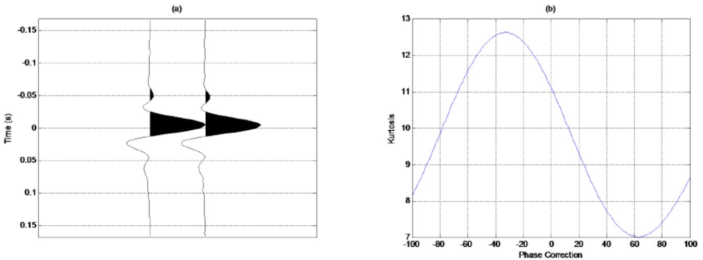
Figure 1. Example of the performance of the code when SNR=20, sparsity=0.8, and constant phase added of  $c=30$ : (a) true wavelet (left) and estimated wavelet (right), (b) kurtosis vs phase correction. Maximum of the kurtosis corresponds to a phase correction of -33 deg.
