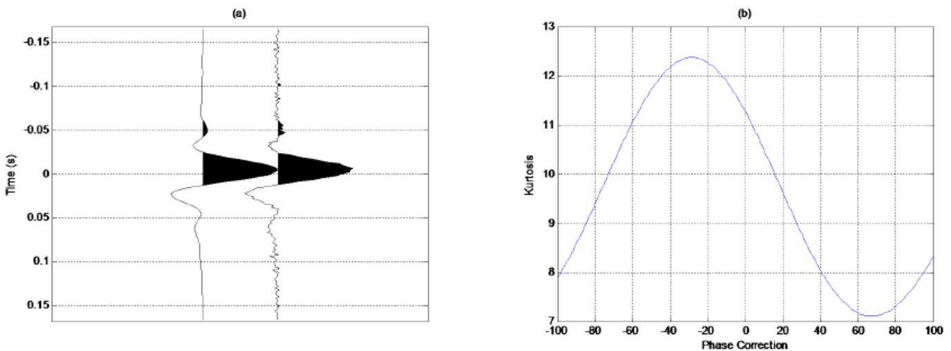
Figure 2. Example of the performance of the code when SNR=5, sparsity=0.1, and constant phase added of  $c=30$ : (a) true wavelet (left) and estimated wavelet (right), (b) kurtosis vs phase correction. Maximum of the kurtosis corresponds to a phase correction of -29 deg.
