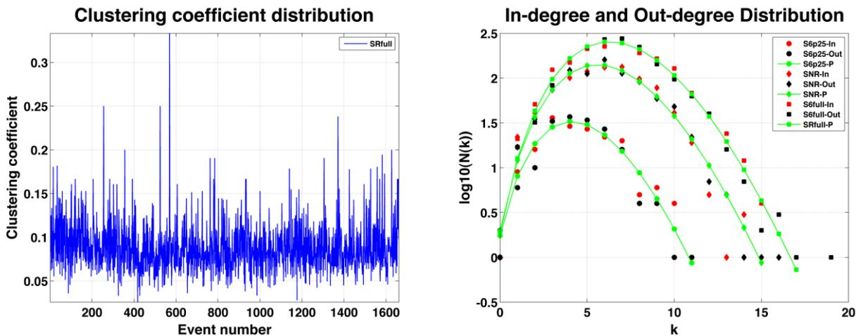
Figure 3: Left: Clustering coefficient of spatio-temporal recurrences for each microseismic event from the stage 6 catalogue; Right: In-degree and Out-degree distributions for three different sets of microscopic events. Also, included in these graphs are the Poisson degree distribution for each data set.
