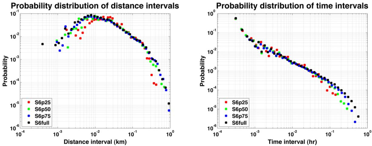
Figure 2: Left: Probability distribution of distance intervals of recurring microseismic events from a hydrofracturing experiment at different times for stage6; Right: Probability distribution of time intervals of recurring microseismic events from a hydrofracturing experiment during different stages
