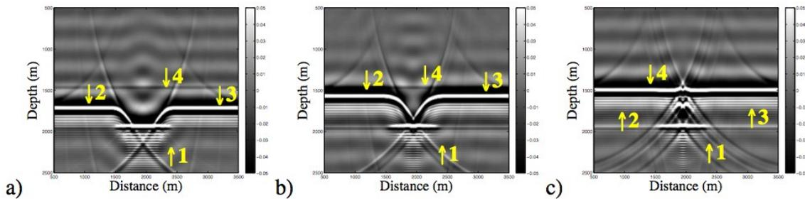
Figure 2: Split-step Fourier migrated seismic sections generated from velocity and synthetic models in Figure 1. Sections(a), (b), (c) capture flattening of hyperbolic events after day  $\tau=1$ , 14 and 28, respectively.
