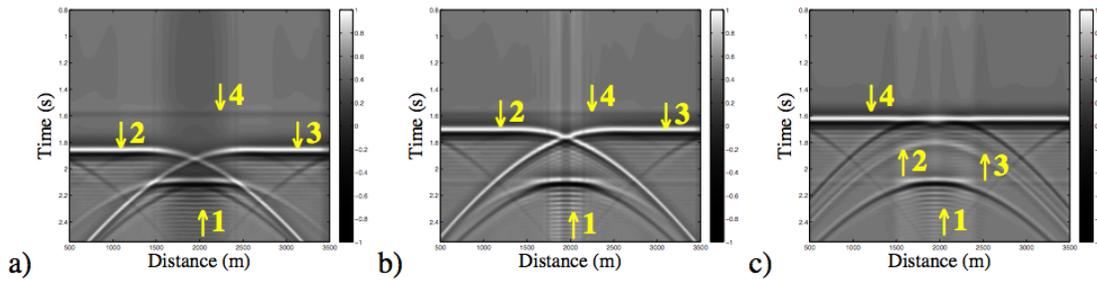
Figure 1: 2D synthetic seismic models generated employing exploding reflector algorithm. Models (a), (b) and (c) show reservoir in time-lapse steps after day  $\tau=1$ , 14 and 28, respectively. Reservoir bottom, top, two waterfrnts are denoted by arrows 1, 4, 2 and 3, respectively.
