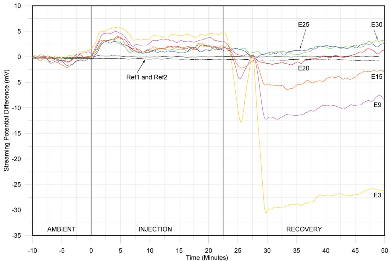
Figure 1: Changes in self potential observed by 6 different surface electrodes prior to, during, and following a constant head injection test at ~44.3 m depth. The selected electrodes show variations in response with respect to distance away from the injection well (colour-coded as in Figure 2). Note the lack of variation in the remote reference (telluric-monitoring) dipoles Ref 1 and Ref2.
