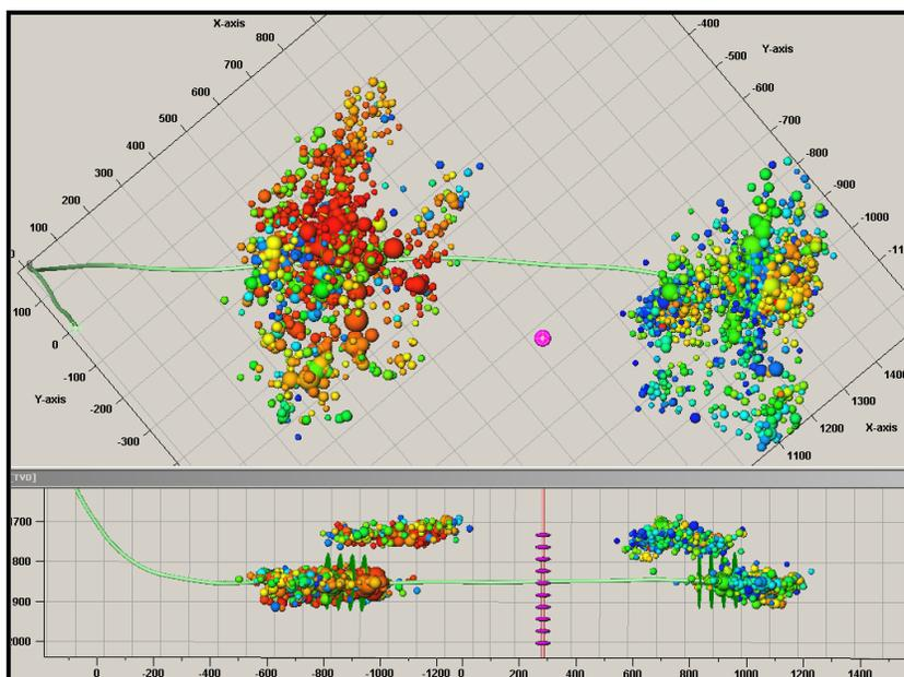
Figure 1: Microseismic Events from stages 1 and 7
