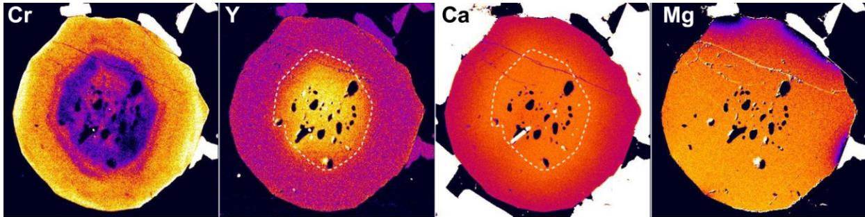
Figure 2: Core-overgrowth compositional domains in garnet porphyroblast revealed using microprobe X-ray mapping. Dashed polygon shows position of Cr-discontinuity.
