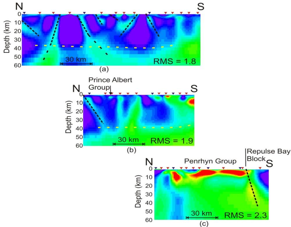
Figure 3: Two-dimensional resistivity models of the MT data. The warm colours (reds) represent low resistivities and the cool colors (blues) resistive regions. The dashed black lines mark fault lines that are mapped at the surface and the yellow dashed line marks the approximate crust-mantle boundary.
