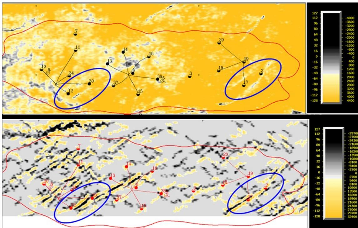
**Figure 1.** Comparison of an amplitude map of single-reflected waves from horizon 1a at the top of a reservoir (top) with that after duplex wave migration for the same horizon (bottom). The red contour shows the oil-bearing area. The most productive wells are outlined with blue ovals.
