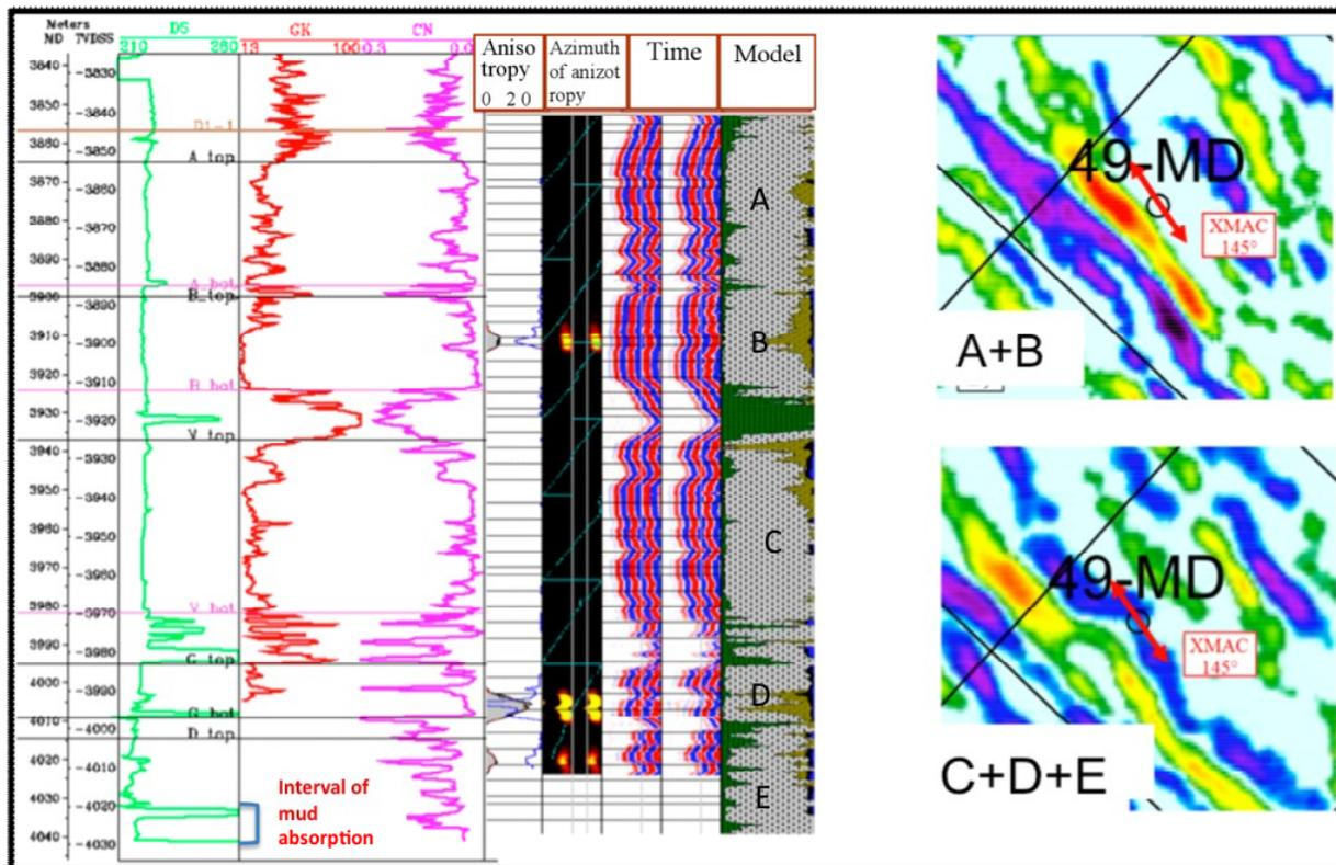
**Figure 2** After production logging in well 49-MD, all the inflow was obtained from an interval within the lower object, where intensive mud absorption occurred while drilling. In the other part of this borehole, according to XMAC data, any significant anisotropy of the rocks is absent (see
