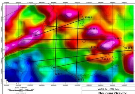
**Figure 1:** Locations of model profiles (thick black lines) overlain on Bouguer gravity map. The thin black line is the mapped boundary of the Aberdeen Sub-Basin, located approximately 100km west of Baker Lake, Nunavut.
