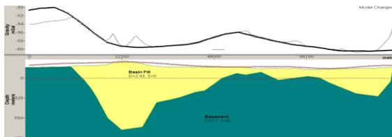
**Figure 2:** GM-SYS Bouguer gravity profile for the EW-1 transect. Top: Observed (heavy dotted line) and computed (thin black line). Bottom: Computed model; basement rocks shown in teal; Thelon Formation (basin fill) shown in pale yellow.
