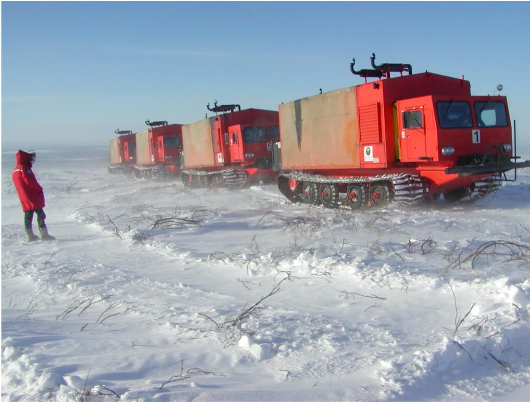
**Figure 2.** Minimizing land, vegetation and wildlife exposure in Mackenzie Valley by acquiring Vibroseis seismic data during the winter.
