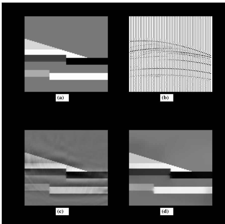
Figure 1: (a) The true layer velocity model. (b) Synthetics data obtained from the single-scattering Born approximation modeling method for a source location at 800 m from the origin. (c) Reconstructed solution using the damped least squares method. (d) Solution obtained using edge-preserving regularization implemented via the total variation (TV) method.
