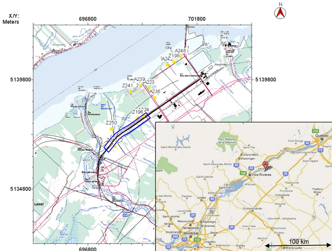
Figure 1: Bécancour area with location of boreholes (yellow dots) and seismic lines (black lines). Blue outline is seismic line n806mg shown in Figure 2. Red lines are roads. Inset: Location of the city of Bécancour (A), Québec, Canada.
