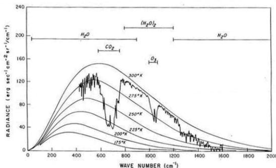
Fig. 4.1 The terrestrial infrared spectra and various absorption bands. Also shown is an active atmospheric emission spectrum taken by the Nimbus 4 IRIS instrument near Guam at 15.1 N and 155.3 W on April 27, 1970.
