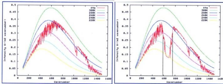
The area above the base of the notch between the two vertical lines represents all of the energy remaining that can be affected by further increases in atmospheric CO<sub>2</sub> concentration above the current level. The question is how much of this remaining energy will be accessed by a doubling of the concentration of atmospheric CO<sub>2</sub> from its current level and what effect this will have on global temperature.
