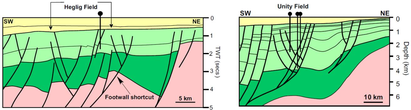
**Figure 4:** Recognizing inversion versus pure extension in Muglad basin, Sudan. A (left): Preserved extensional geometry, interpreted inversion fairway (arrow brackets) and setting for the Heglig oil field. Redrawn from interpreted seismic section in Mohamed et al. 2000. B (right): Cross section showing preserved extensional geometry, possible subtle inversion and setting of the Unity oil field. After Giedt (1990).
