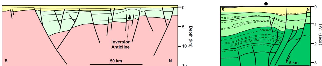
Figure 3: Inversion examples. A (left): Cross section showing inversion in Bongor Basin, more notable in northern part of basin. After Genik (1993). B (right): Inversion structure and petroleum trap in Doseo basin. Redrawn from interpreted seismic section in Genik (1993).
